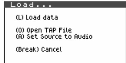
The first source of recordings is the audio (EAR) socket. The source can also be a TAP file stored on a memory card, to select a file it is necessary to use (**O**)**pen TAP File**.
